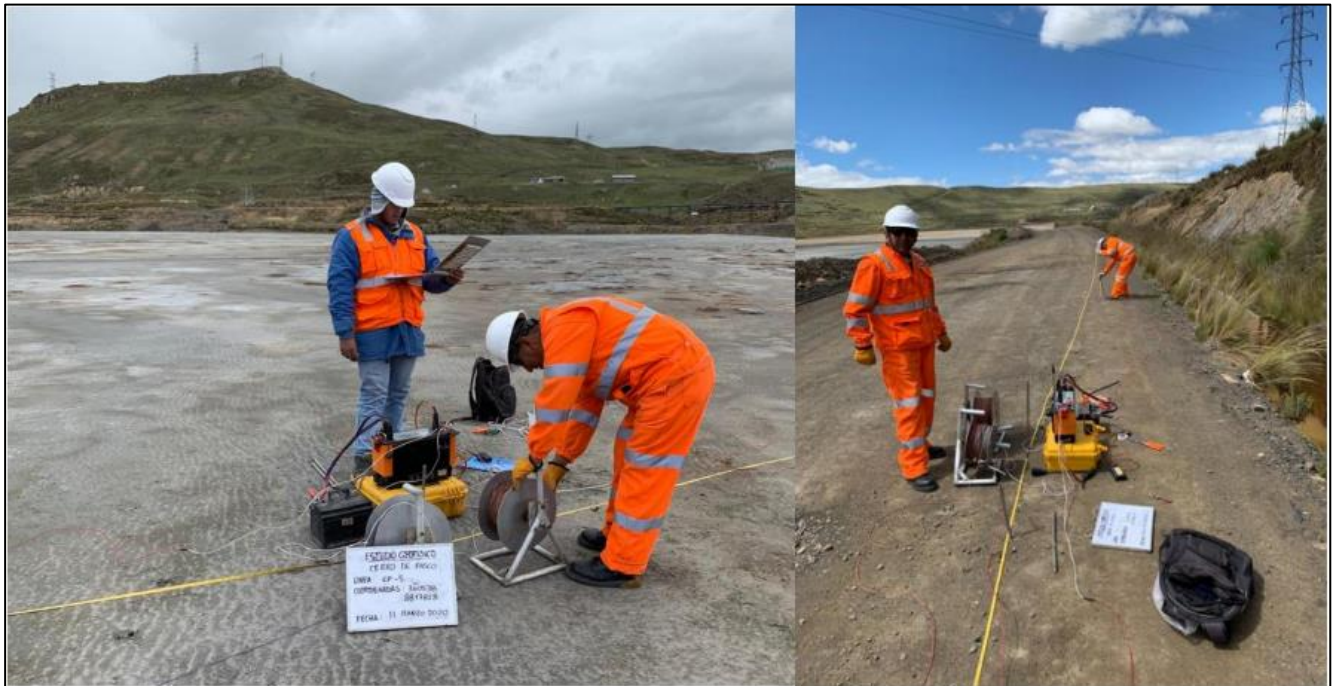
Figure 9-1: JCI carrying out the VES geophysical survey
