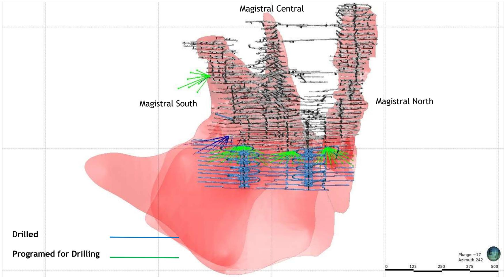
**Figure 3:** Infill drill program with drilled and programmed holes
