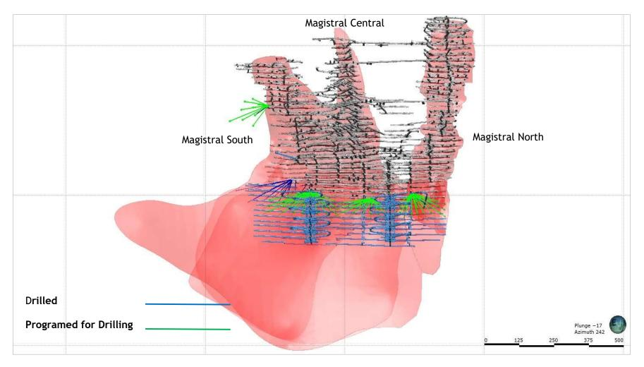
Figure 3: Infill drill program with drilled and programed holes
