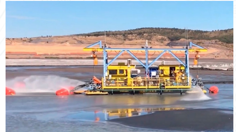
Example of Pump Pontoon for Tailings Extraction
